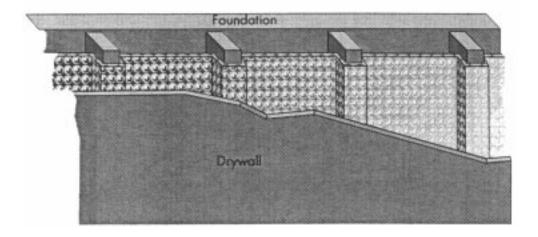
1) Fasten 2x4 wall against concrete foundation using usual methods.
